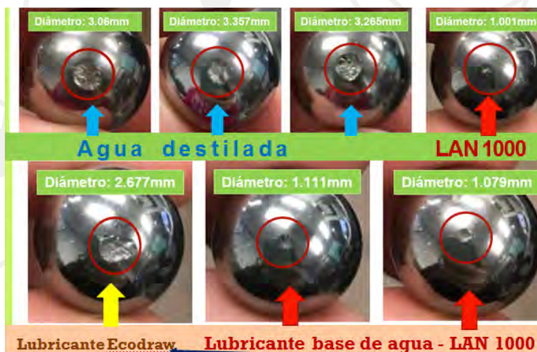
Figure 1 –Tribological test with four balls.
