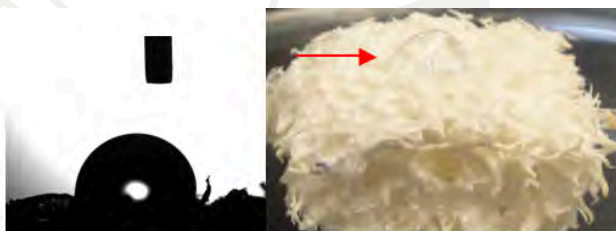
Figure 1. A water droplet as a spherical shape trace on the surface of the modified luffa sponge
