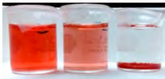
Figure 2. Original solution (left), solution degraded by TCM (center) and solution degraded by TNM (right).
